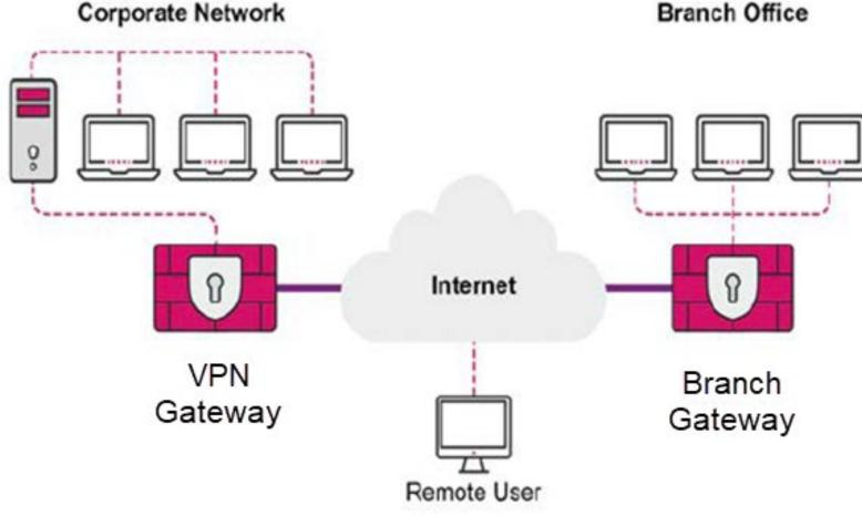
**IPSec VPN tunnels** can be established between two Security Gateways to securely pass traffic between hosts behind these Security Gateways by encrypting and authenticating it.
