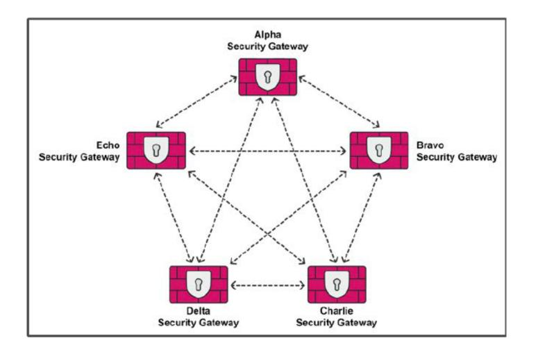
Any VPN Gateway in the Mesh community can establish a direct VPN tunnel with any peer Gateway in the Mesh community.
